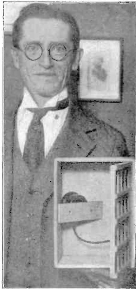
(Photonews) EDWARD A. LE FEBRE , of Astoria, L. I., is shown with a loud-speaking unit using walls of box as reflector.
